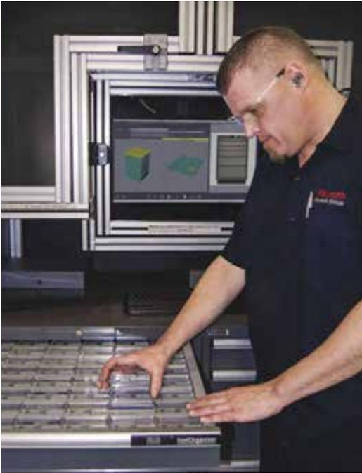
Once the tools are designed, the Zoller Tool Organizer enables Bosch Rexroth's tool group to know the exact location of each and every tool or component. Interfaced directly to Zoller stock management, Tool Organizer helps keep track of tool components and other indirect materials.
