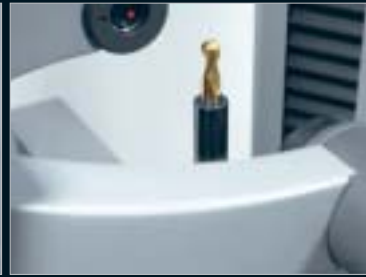
00:16 Automatic measurement of tool cutting edge
