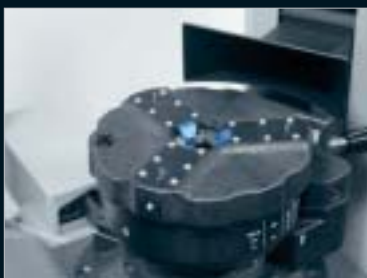
00:32 Induction coil moves automatically into position, heating starts
