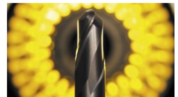
Holistic measurement of cutting tools in transmitted and incident light
